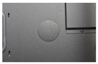
6. To use Tech Station install rubber feet in each corner of the motherboard tray.
